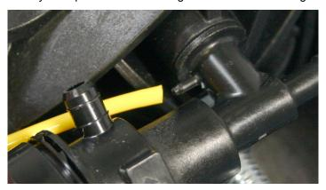
FIGURE 8-11: PRESSURE LINE REMOVAL
