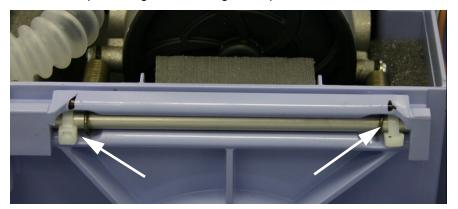
FIGURE 8-22: MOUNTING ROD TIE WRAPS
