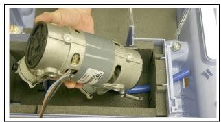
FIGURE 8-24: COMPRESSOR REMOVAL
