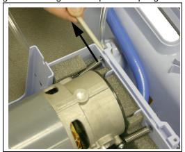
FIGURE 8-23: MOUNTING ROD REMOVAL
